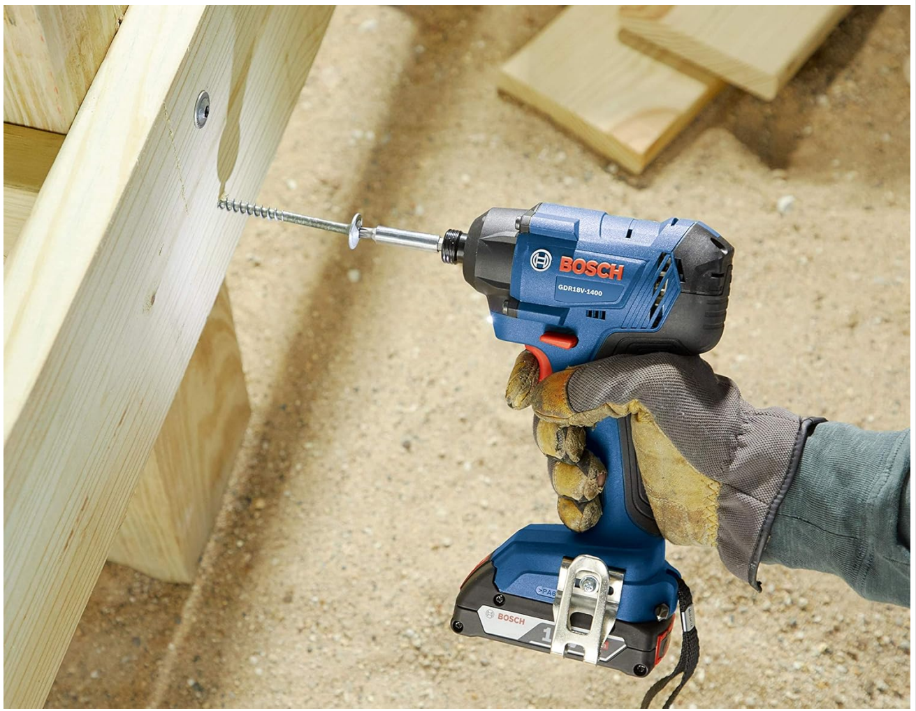
Figure 5.1: Driving a screw into wood using the impact driver.
