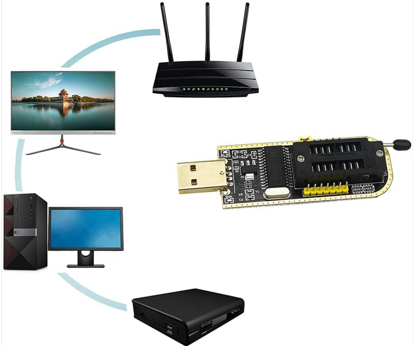
Figure 6: The CH341A Programmer can be used to backup, erase, burn, and verify various software on devices such as routers, computers, and set-top boxes.
