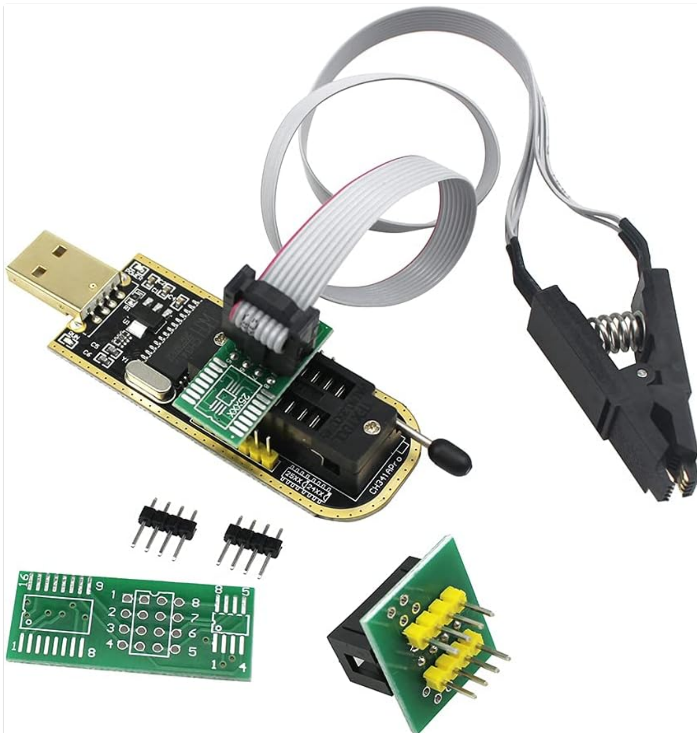
Figure 4: Example of the CH341A Programmer connected to the SOP8 Test Clip and a converter board.
