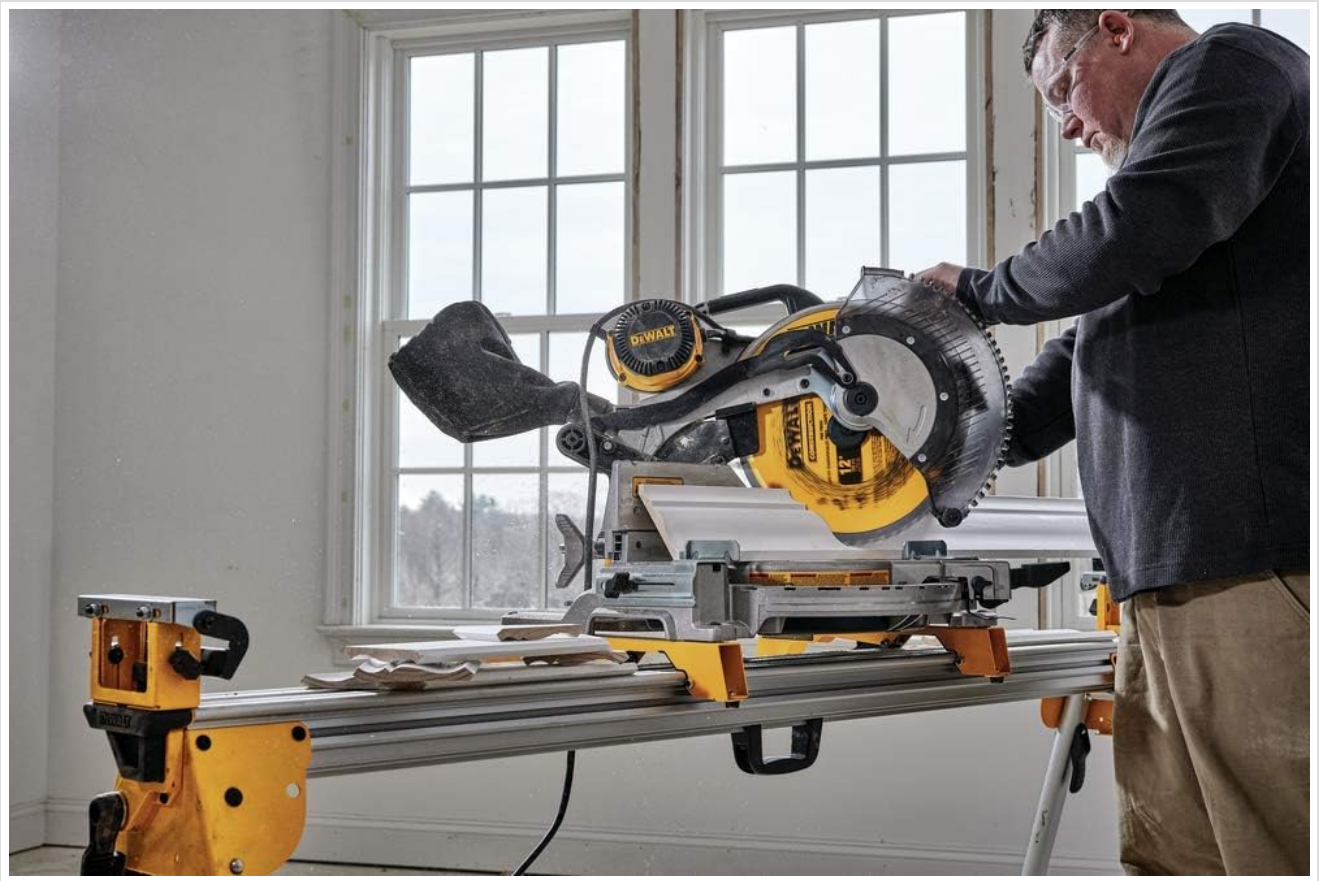
Figure 3.4: The miter saw positioned for a bevel cut, demonstrating its versatility.
