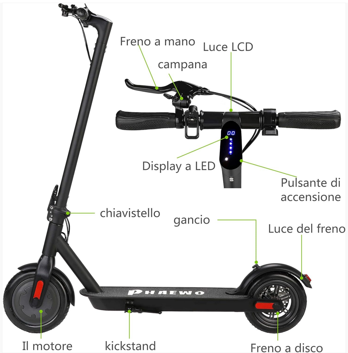
Image: A detailed diagram of the Phaewo X9 Electric Scooter, highlighting its key components with labels in Italian, which include Handbrake, LCD Light, LED Display, Power Button, Bell, Key Lock, Hook, Brake Light, Motor, Kickstand, and Disc Brake.
