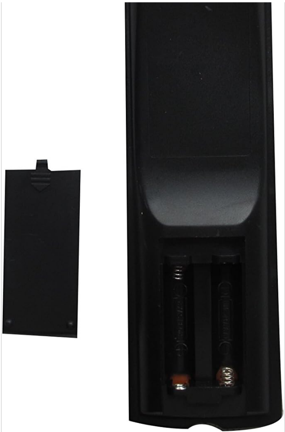
Image showing the back of the remote control with the battery cover removed, revealing two AAA battery slots for installation.
