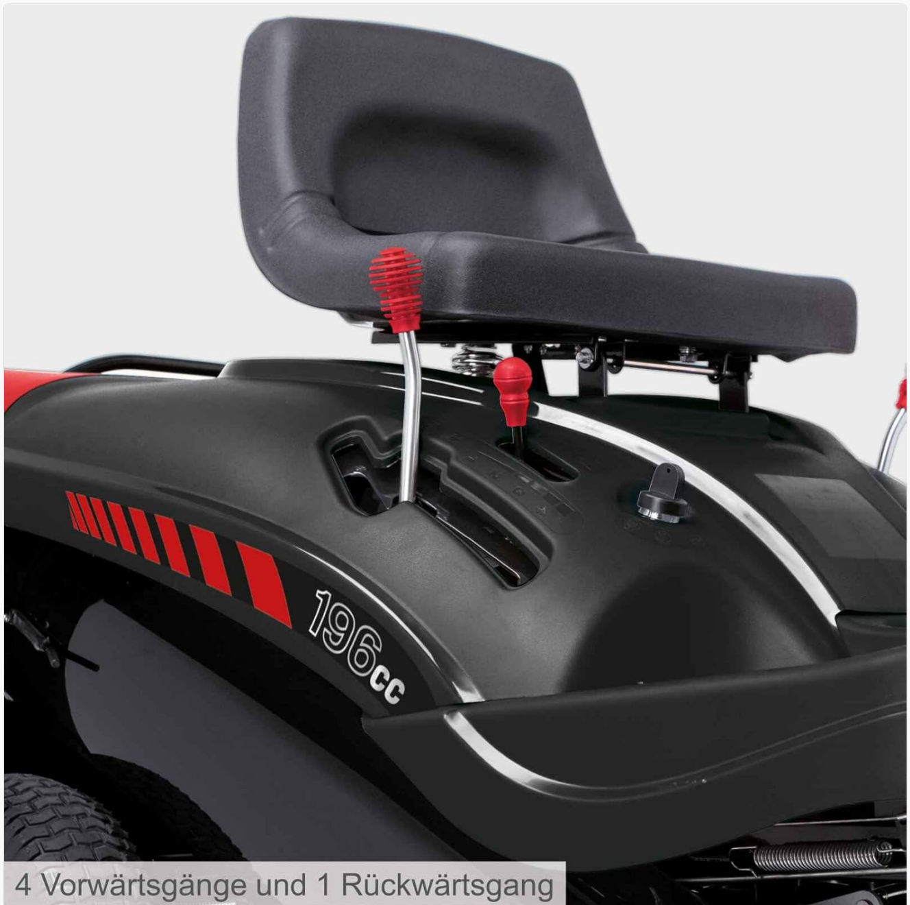
Image 5.1: Close-up of the gear selection levers, indicating 4 forward speeds and 1 reverse speed.
