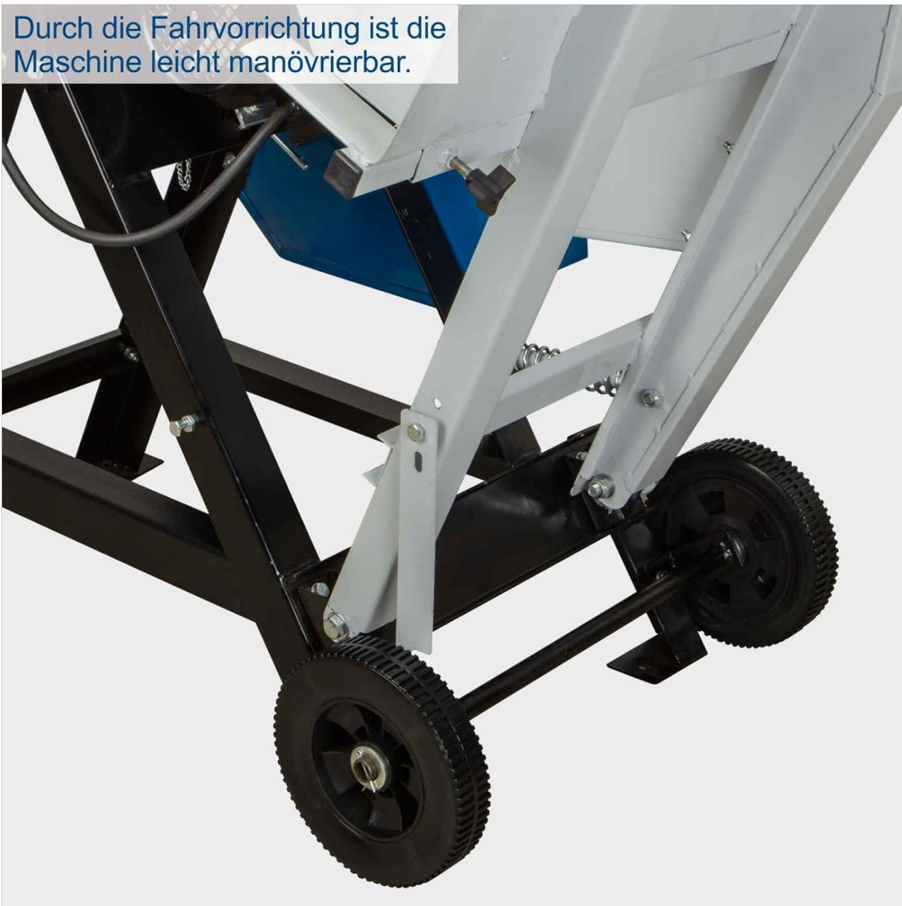
The integrated wheels on the Scheppach HS510 tilting saw allow for easy maneuverability and transport of the machine around the workspace.
