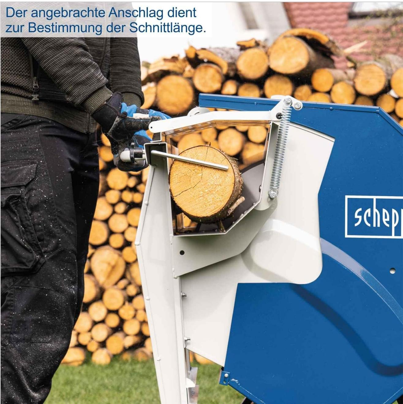
This image shows a user operating the Scheppach HS510 tilting saw. A log is placed in the cradle, and the adjustable stop is utilized to ensure precise and consistent cutting lengths.
