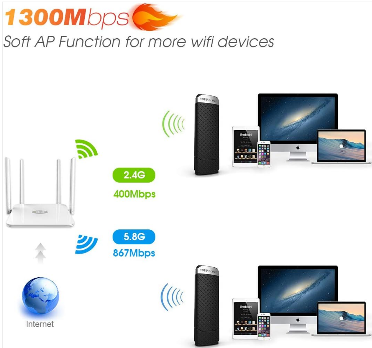
Image: Illustration of the Soft AP function, demonstrating how the adapter can create a Wi-Fi hotspot for multiple devices on both 2.4GHz and 5.8GHz bands.
