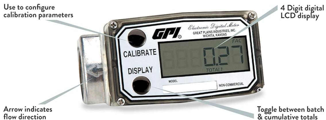
Figure 3.2: Annotated diagram highlighting key components and functions: "CALIBRATE" button for configuration, "DISPLAY" button to toggle totals, arrow indicating flow direction, and the 4-digit digital LCD display showing "TOTAL1" (cumulative) and "FAC" (batch) readings.
