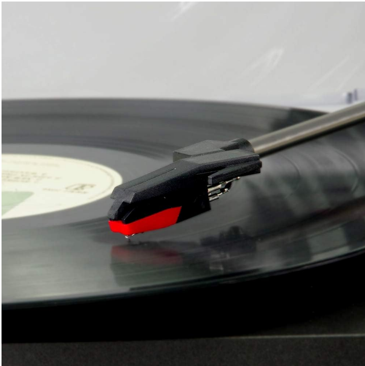
Figure 2.2: Detailed view of a single replacement needle, highlighting the stylus tip.
