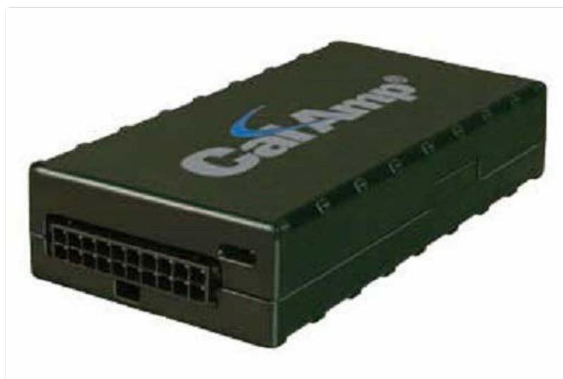
Image 1: The CalAmp LMU-2630 GPS Tracker unit, a compact dark-colored device with a multi-pin connector on one end and the 'CalAmp' logo on top.
