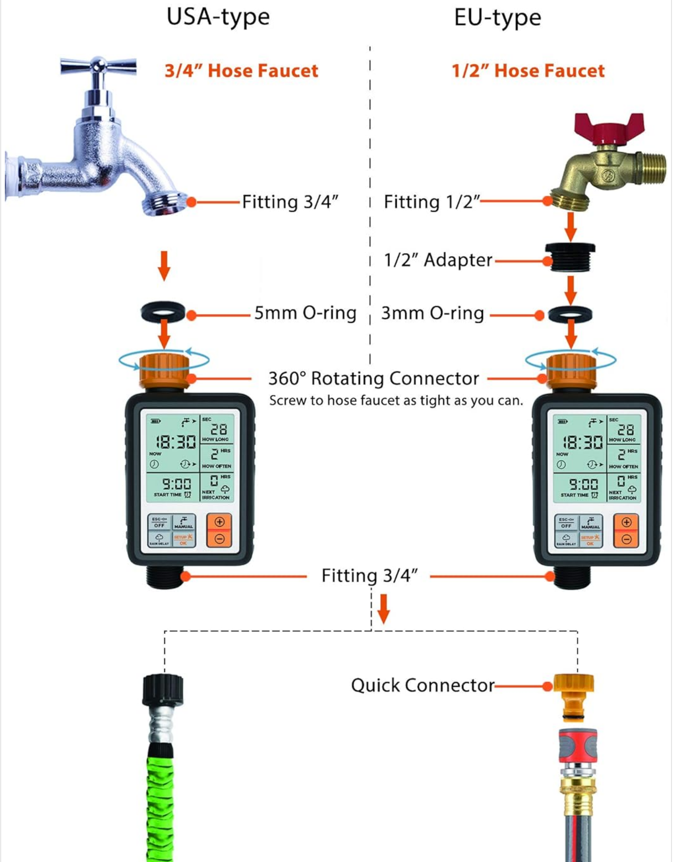
Figure 4: Quick Installation Diagram for Kazeila watering timer, showing connection to USA-type (3/4 inch hose faucet) and EU-type (1/2 inch hose faucet with adapter) faucets, including O-rings and 360-degree rotating connector.
