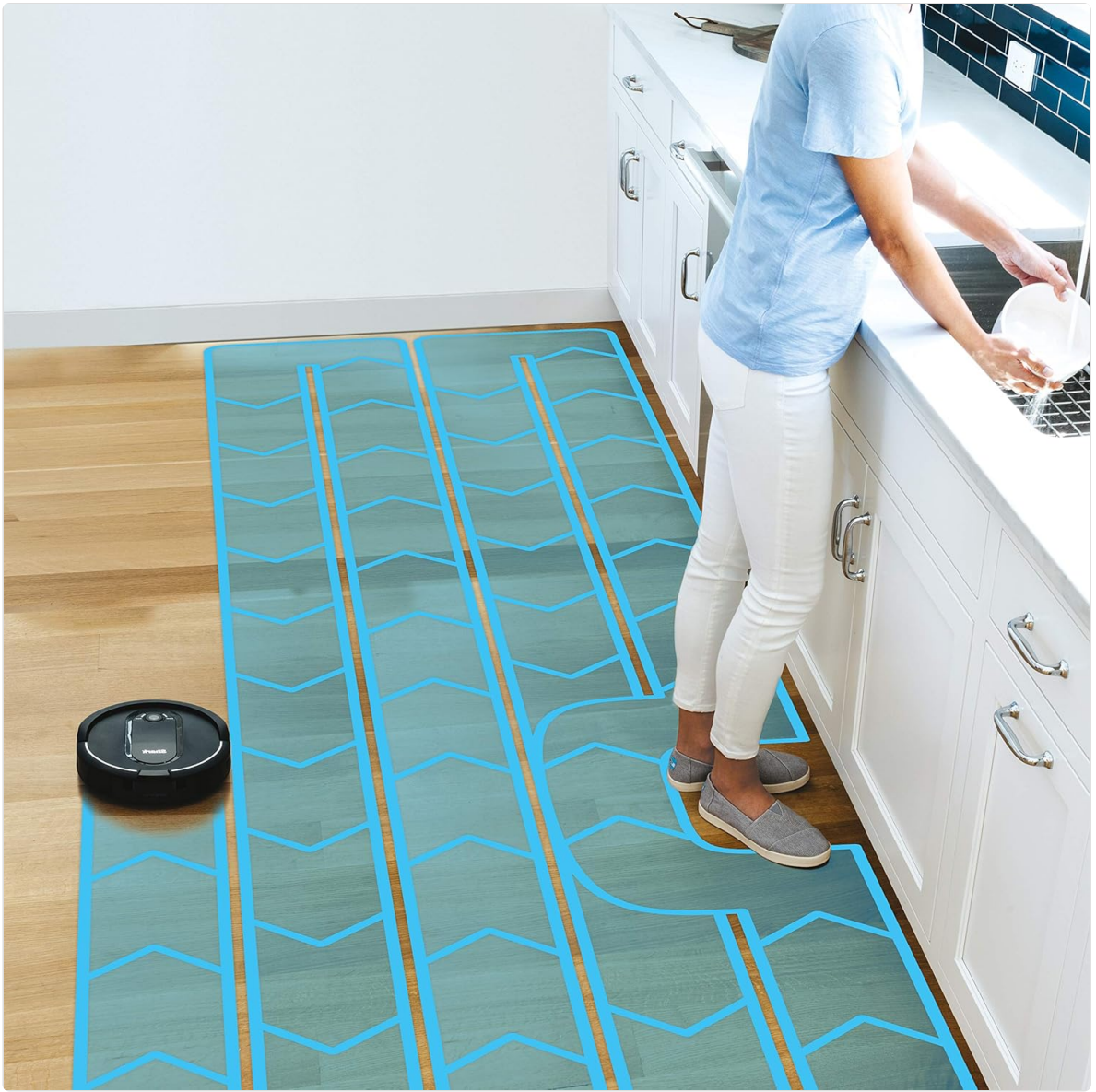
Image: The Shark IQ Robot Vacuum navigating a kitchen floor, with blue lines overlaid to illustrate its mapping process and systematic cleaning pattern.
