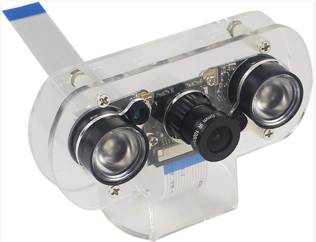
Image: The camera module fully assembled inside its clear acrylic protective case, showing the lens and IR lights.
