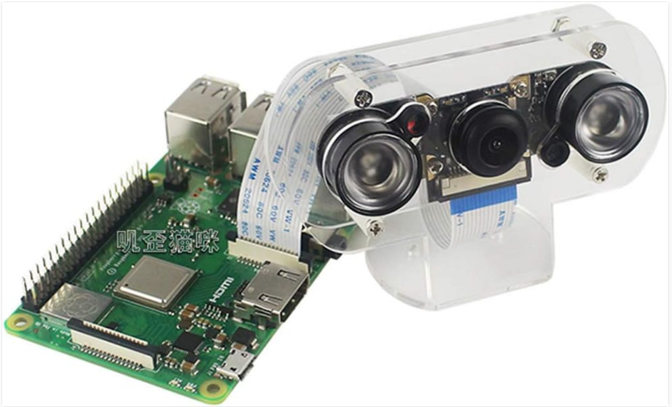
Image: The assembled camera module connected via its ribbon cable to a Raspberry Pi single-board computer.
