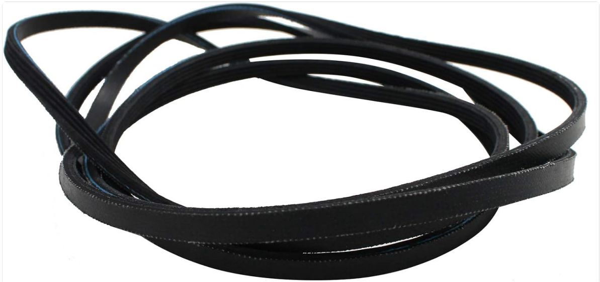
Figure 2: A close-up view of the replacement dryer drum belt, showing its flexible and ribbed construction. The ribbed side must make contact with the motor pulley for proper operation.
