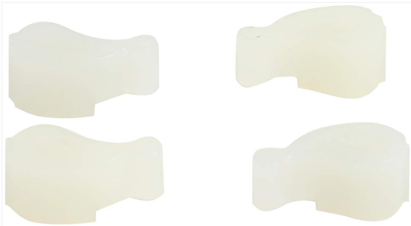
Figure 1: UpStart Components 80040 Washer Agitator Dogs. This image displays four individual washer agitator dogs, which are small, white, plastic components. These parts are crucial for the agitator's function in a washing machine, allowing it to rotate in one direction to move clothes while slipping in the other direction.
