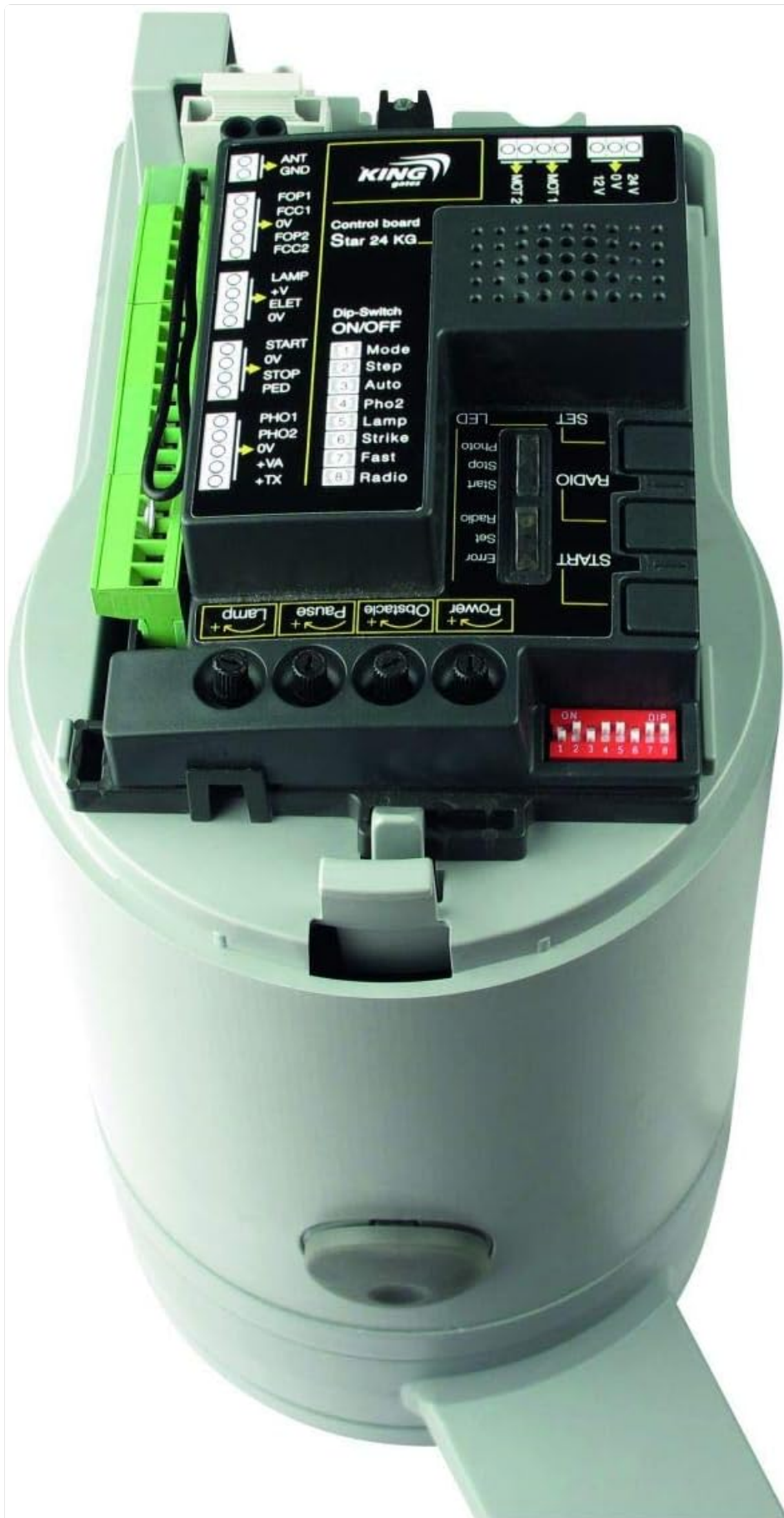
Image: Internal view of the King Gates Mini Modus master unit, showing the control board and wiring terminals.
