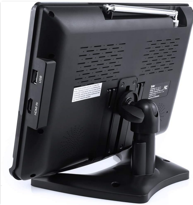
Image: Rear view of the Tyler TTV706 TV, highlighting the HDMI and USB input ports on the side.
