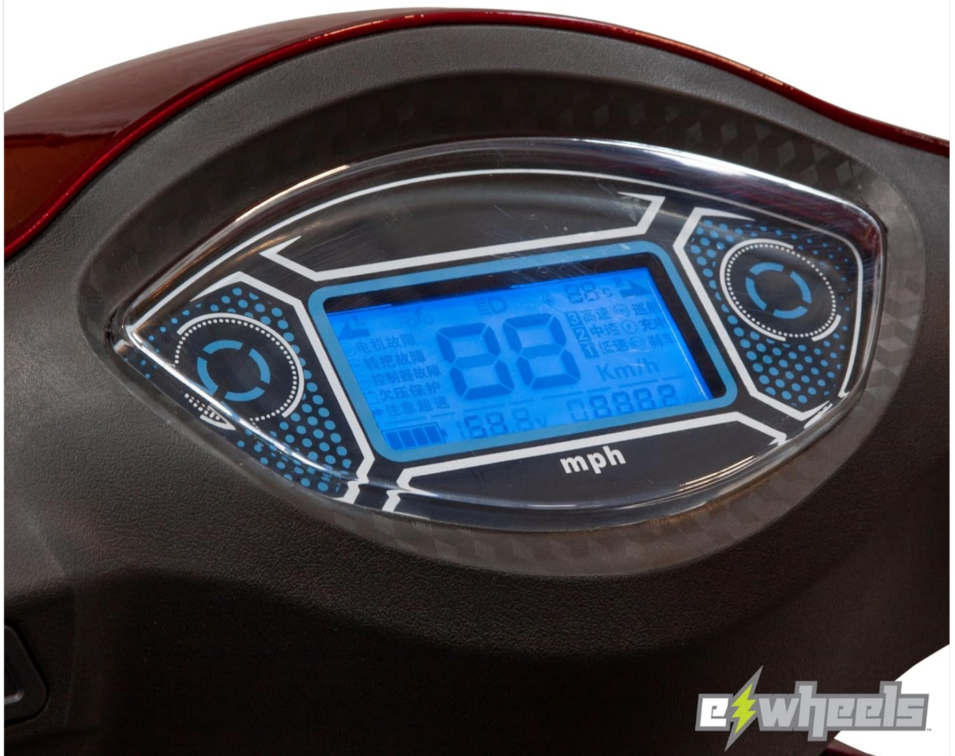
Image: A detailed view of the EW46 scooter's easy-to-read LED display, showing speed, battery level, and other operational indicators.
