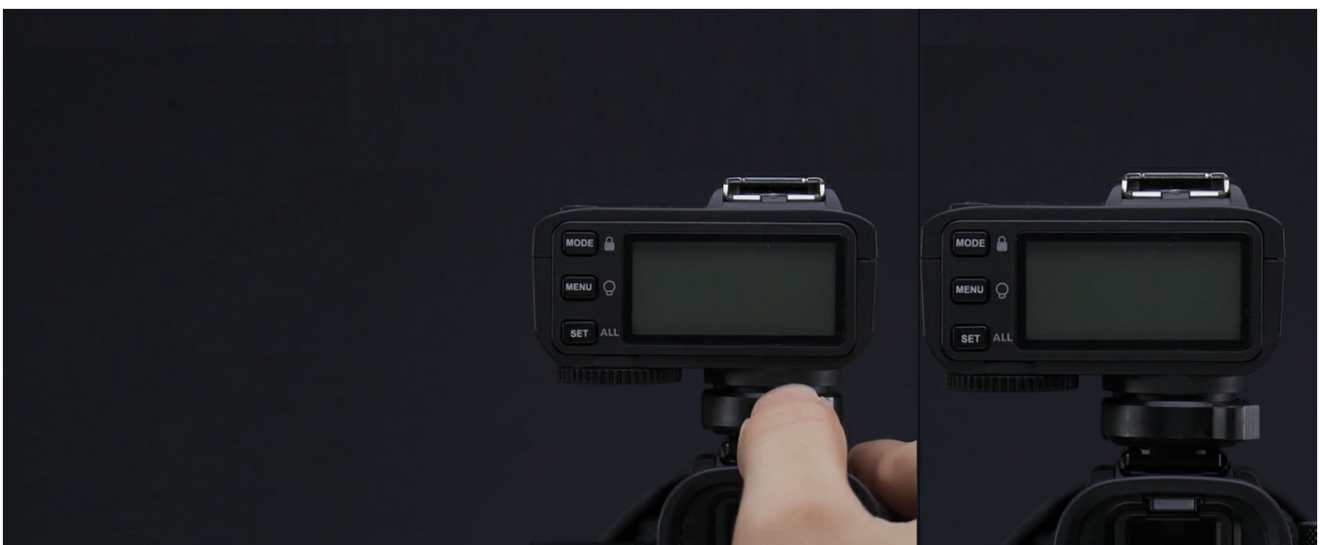
Figure 3.3: Close-up of the X2T-S hot shoe locking mechanism, ensuring secure attachment to the camera.
