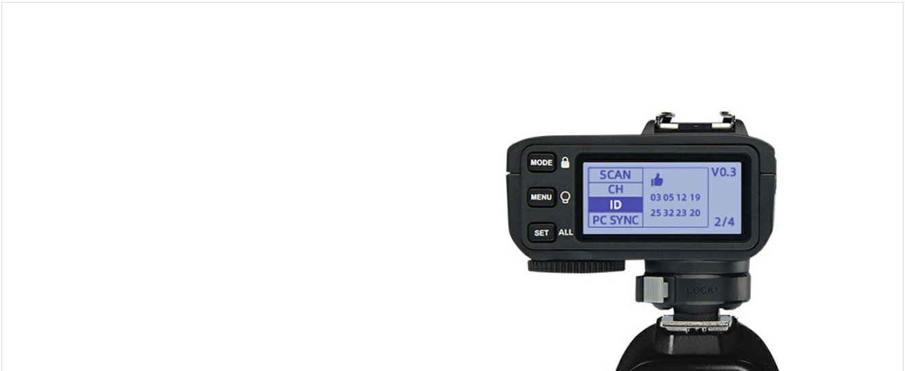
Figure 3.4: The X2T-S display showing options for scanning channels, setting channels (CH), and wireless ID (ID).
