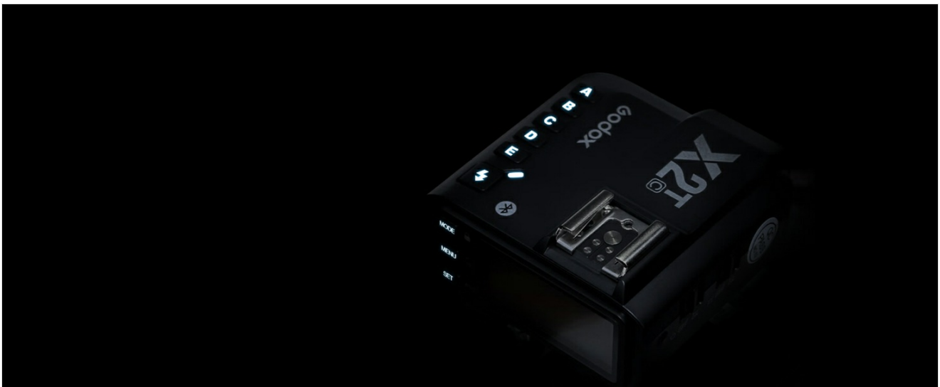
Figure 4.2: The Godox X2T-S with its group selection buttons illuminated, indicating active groups.
