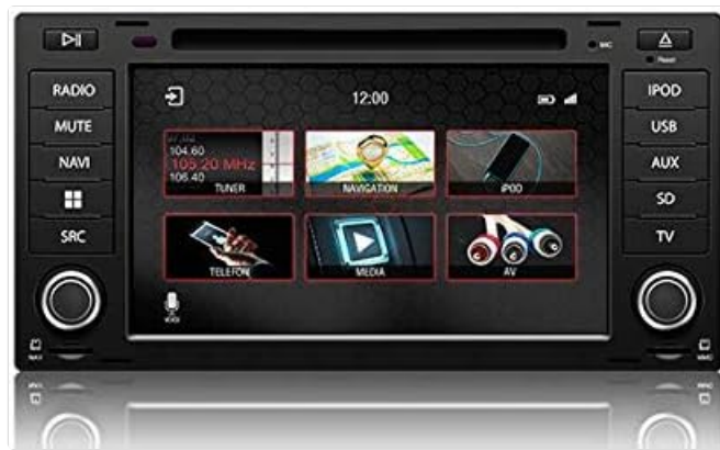
Figure 4.1: The main menu screen displaying various function icons such as Radio, Navigation, Telephone, Media, and AV input.
