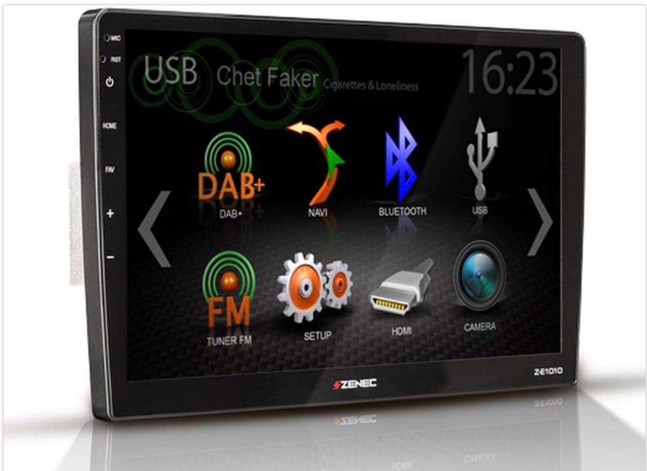
Figure 5.1: Zenec Z-E1010 Infotainment System main screen. This image illustrates the primary user interface of the Zenec Z-E1010 Infotainment System. The screen shows various selectable icons for core functions such as USB media playback, DAB+ digital radio, navigation, Bluetooth connectivity, FM radio, system setup, HDMI input, and camera view. The current time '16:23' is visible in the top right corner, and 'Chet Faker - Cigarettes & Loneliness' is displayed as the currently playing track via USB.
