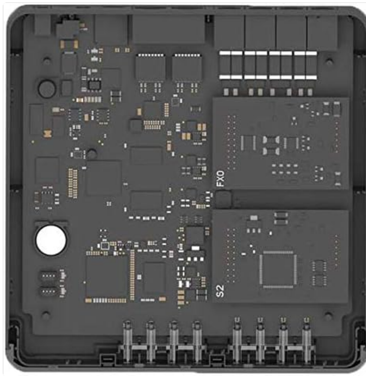
Image: Internal view of the Yeastar S20 circuit board, illustrating the modular design with slots for expansion cards like FX0 and S2 modules.
