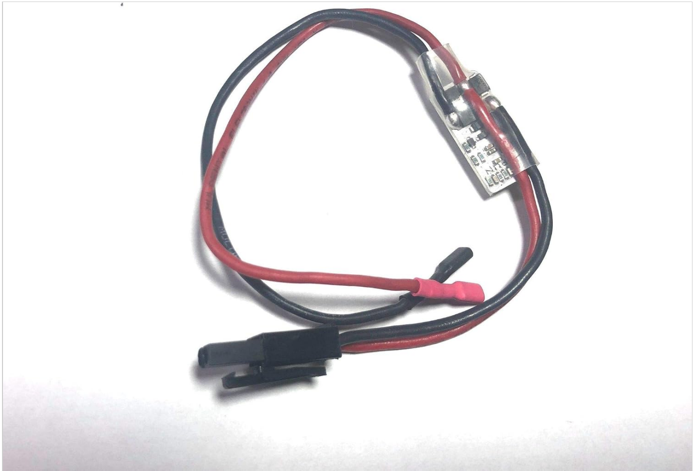
Image 1: The PERUN ETU++ wiring harness, featuring a Tamiya connector for battery connection. This unit replaces the stock G&G ETU board.
