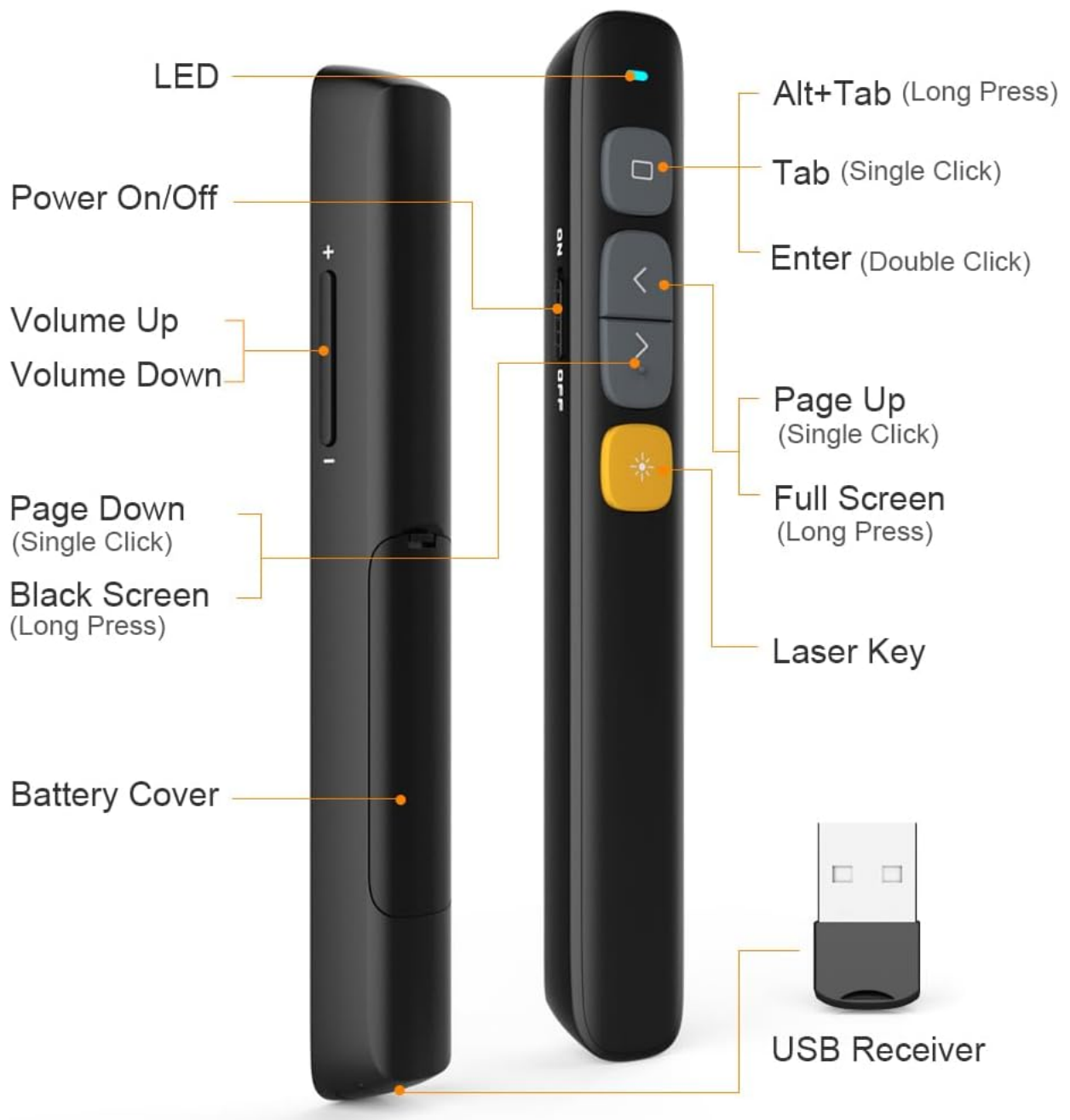
Image 3.1: Detailed button functions of the Norwii N29 remote.
