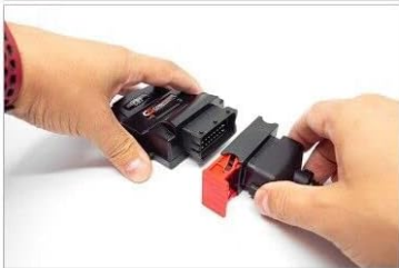
Image 4.2: Visual sequence demonstrating how to connect the ChipPower GS1 module to the vehicle's sensor.
