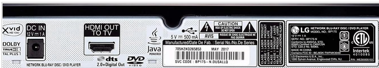
Image: Rear panel of the LG BP175 player, highlighting the HDMI output port.
