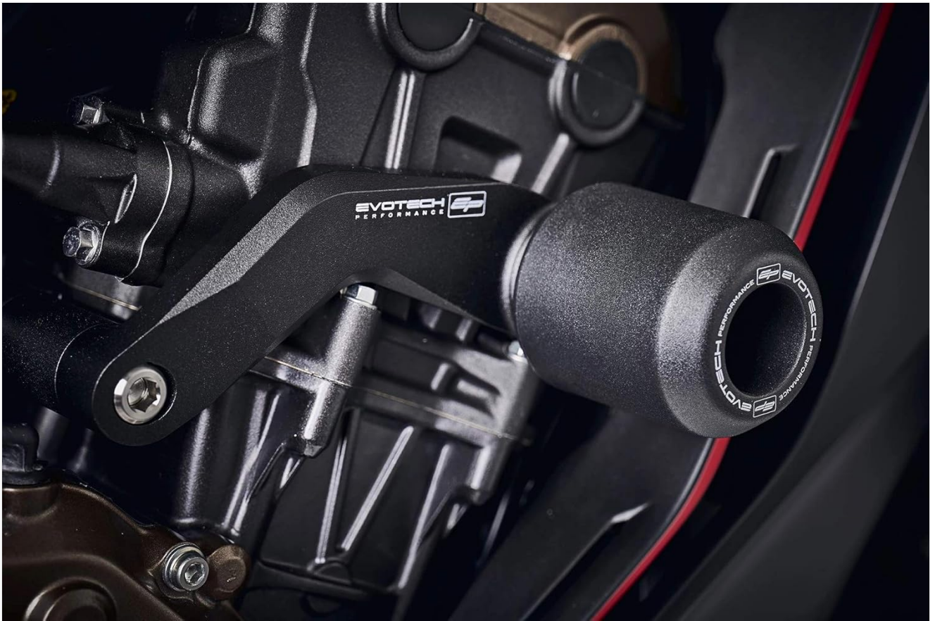
Figure 5.2: Right side EVOTECH frame slider installed. Similar to the left side, this image shows the right frame slider mounted, highlighting its integration with the motorcycle's frame and engine components.
