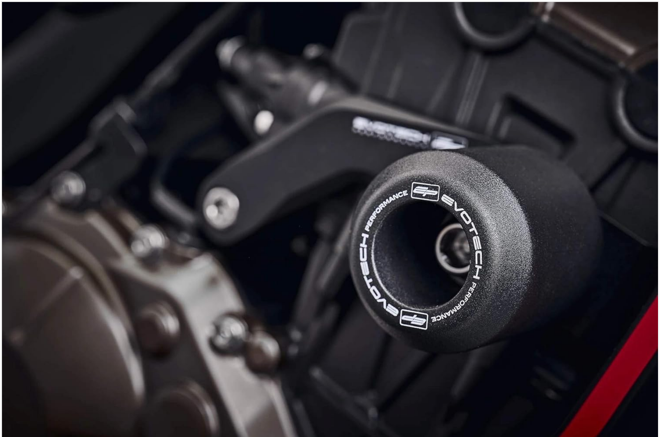
Figure 5.1: Left side EVOTECH frame slider installed. This image provides a detailed view of the left frame slider securely mounted to the motorcycle's engine block, showcasing the bracket and the slider bobbin in position.
