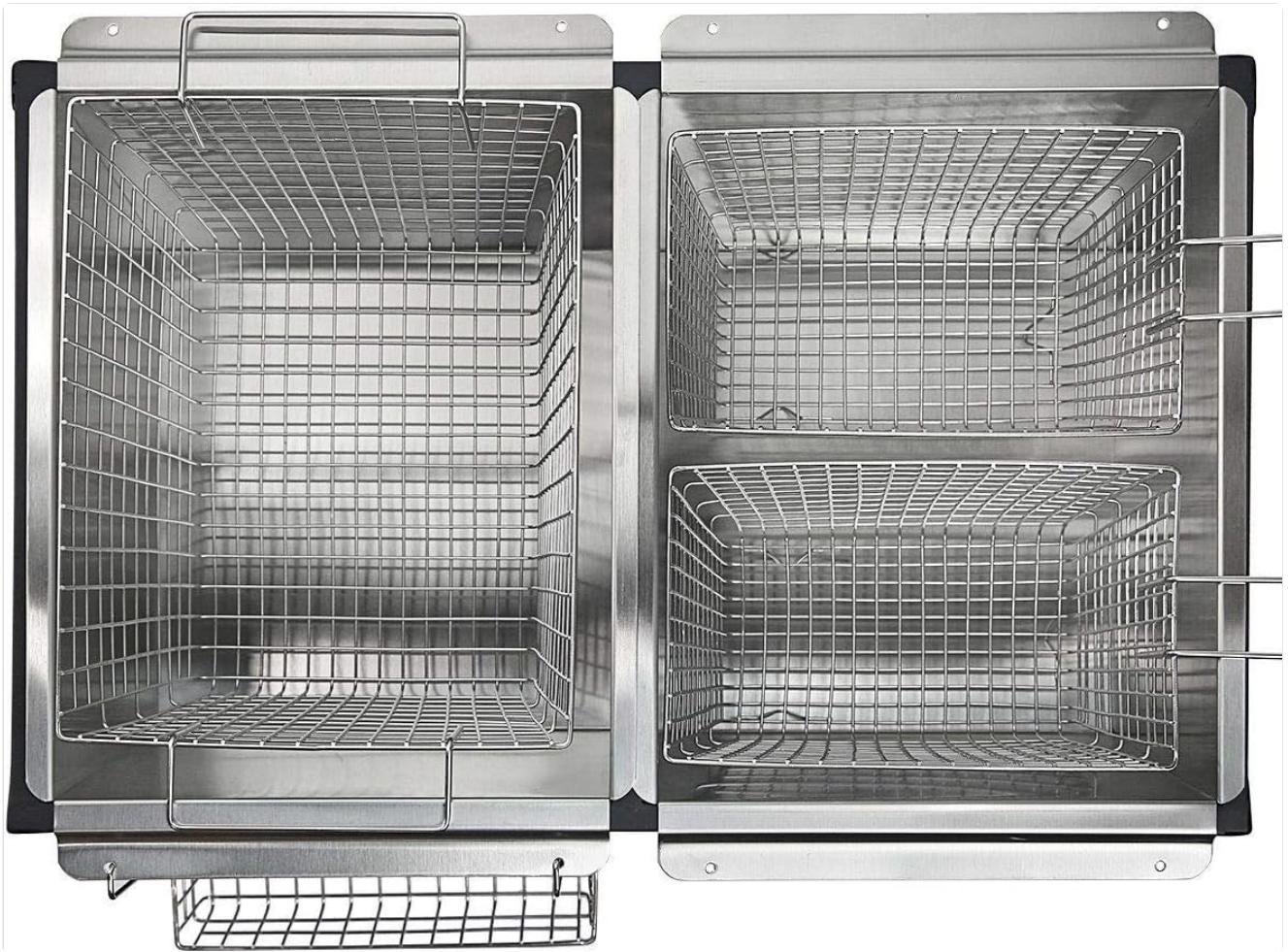
Figure 2.2: Top view illustrating the triple basket configuration within the two fry pots.
