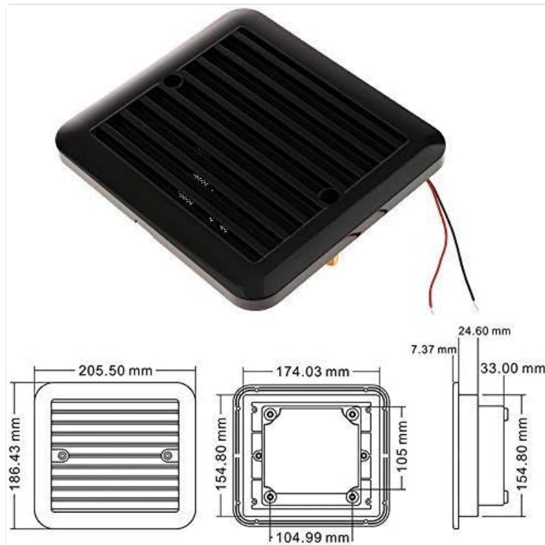
Figure 3: Detailed dimensions of the MASO Exhaust Port Fan.
