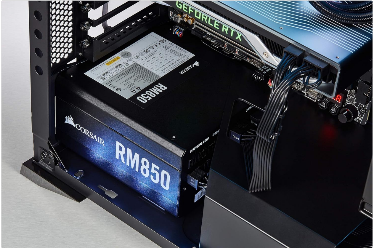
Image 2.1: The RM850 power supply installed within a computer case.
