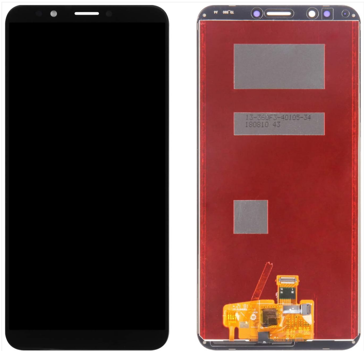
Image showing the front (display side) and back (flex cable side) of the SRJTEK screen replacement unit. Observe the delicate flex
