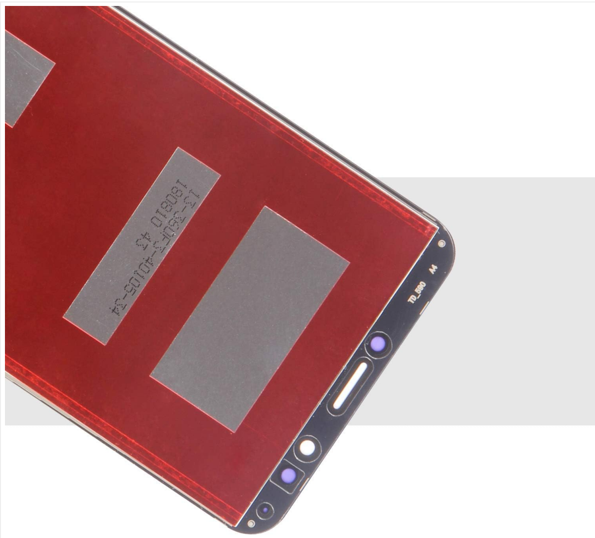
Angled view of the top portion of the screen's back, showing the camera and sensor cutouts, and the delicate flex cable routing. Handle with care to avoid damage.
