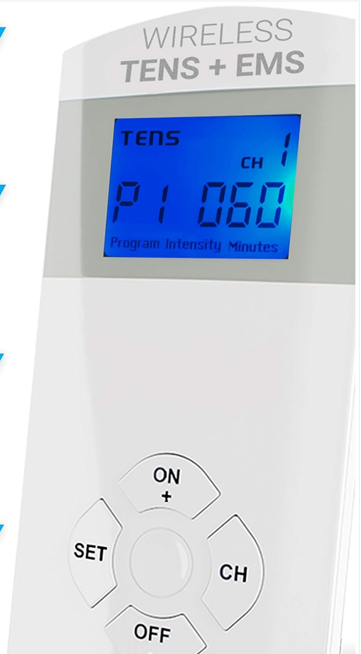
Figure 6.1: A close-up view of the iReliev remote control, showing the digital display with program (P1), channel (CH 1), and treatment time (060 minutes) settings. The control buttons for ON/+, OFF/-, SET, and CH are also visible.
