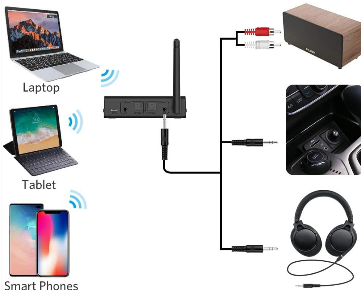
Image: Nulaxy BR04 RX Mode connection diagram.
