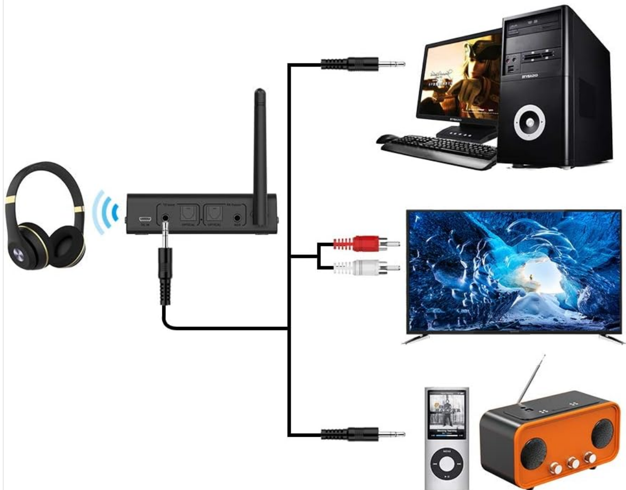
Image: Nulaxy BR04 TX Mode connection diagram.
