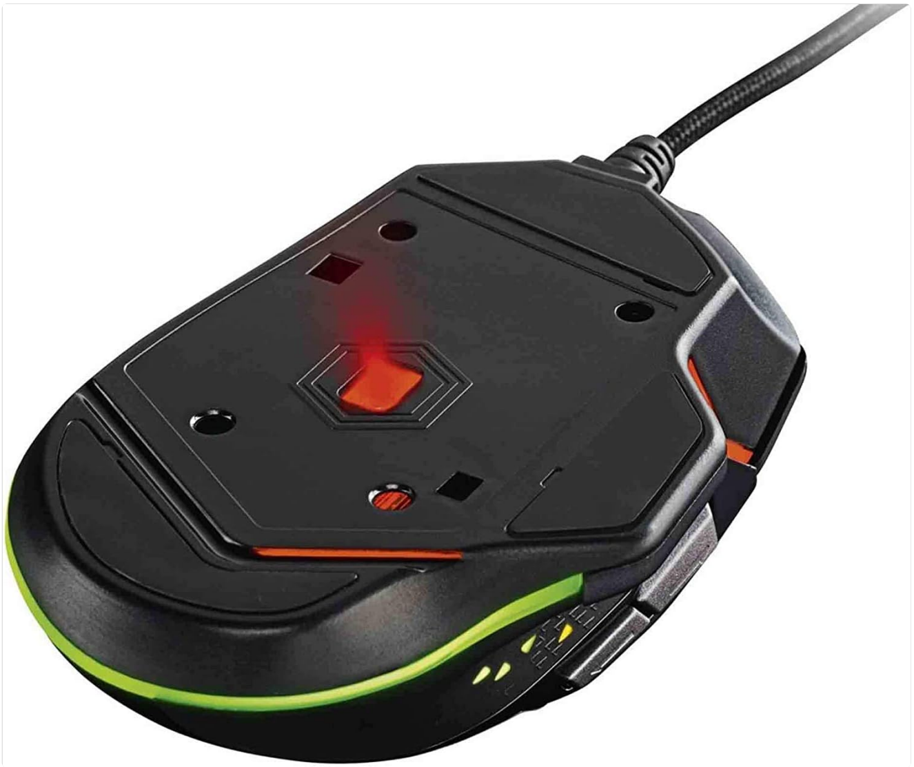
Figure 6.1: Underside of the SilverCrest SGM 4000 A1 Gaming Mouse, showing the optical sensor.
