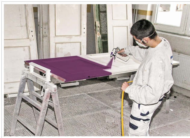
Image: A person demonstrating the use of an airless sprayer with a Wagner nozzle to apply purple paint to a door, showcasing proper technique.
