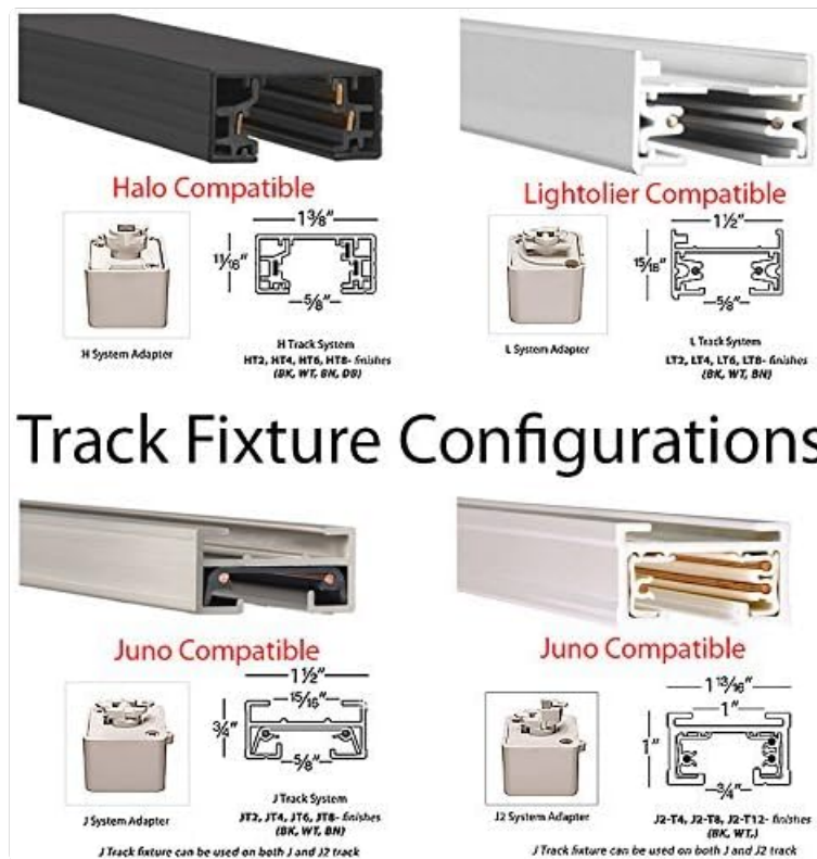
Image 4.1: Track Fixture Configurations and Compatibility.
