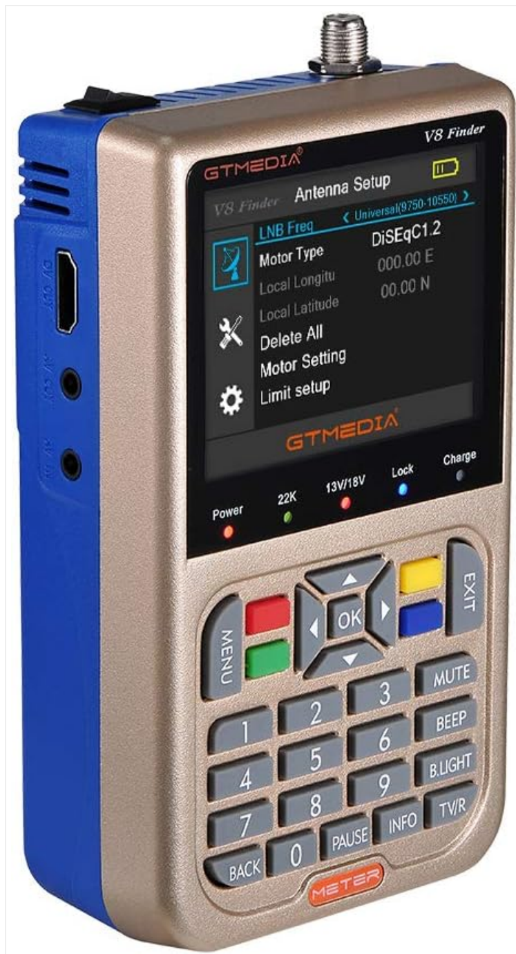
Image 4.1: Front view of the GTMEDIA V8 Finder, showing the LCD screen and control buttons.
