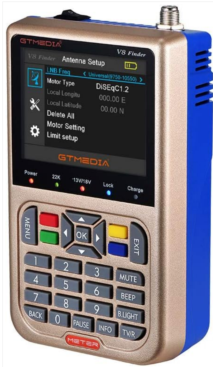
Image 6.1: The "Antenna Setup" screen, showing options for LNB frequency, motor type, and DiSEqC settings.
