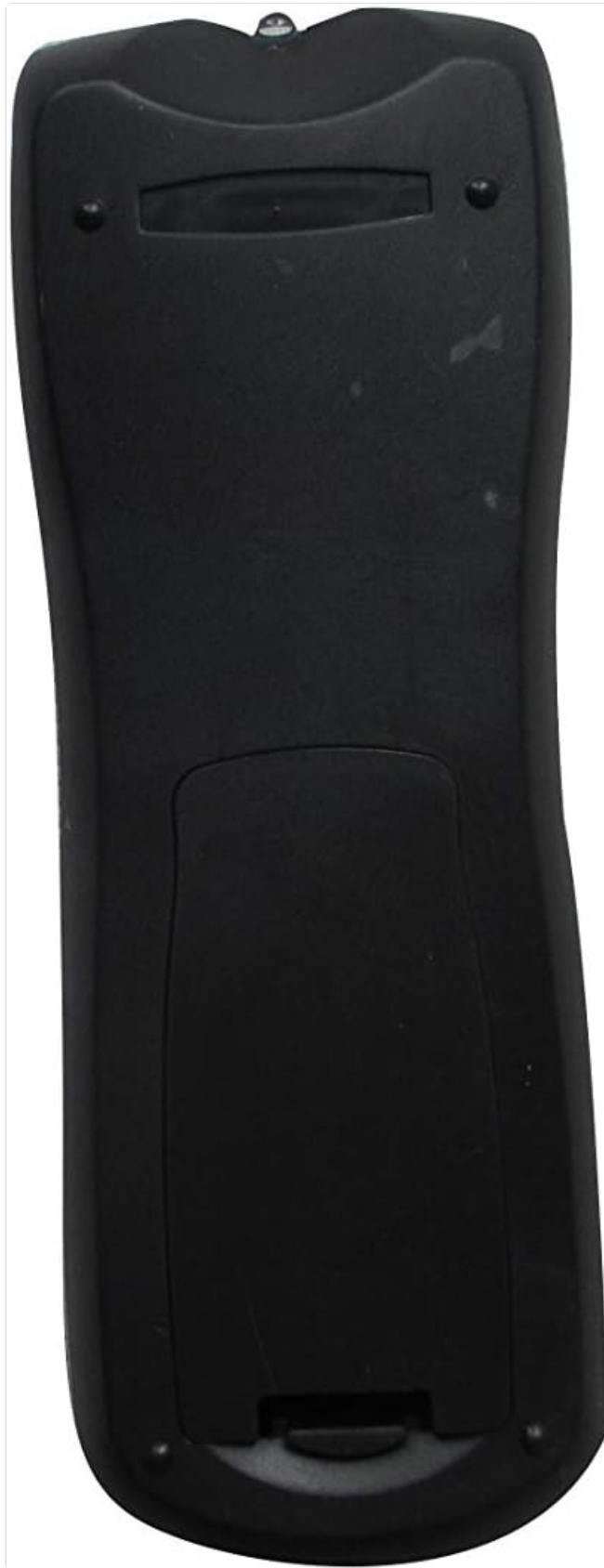
Figure 2: Back view of the remote control, illustrating the battery compartment.
