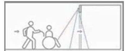
Figure 3.2: The sensor in operation, illustrating its microwave detection field. The red overlay indicates the active sensing area, demonstrating its ability to track motion for automatic door applications.
