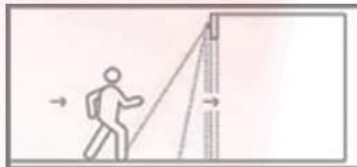
Figure 3.2: The sensor in operation, illustrating its microwave detection field. The red overlay indicates the active sensing area, demonstrating its ability to track motion for automatic door applications.
