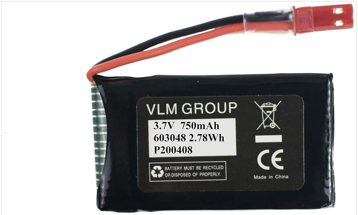
Figure 2.1: Close-up view of the VLM 3.7V 750mAh Li-Po Battery, showing its specifications and proper disposal instructions.
