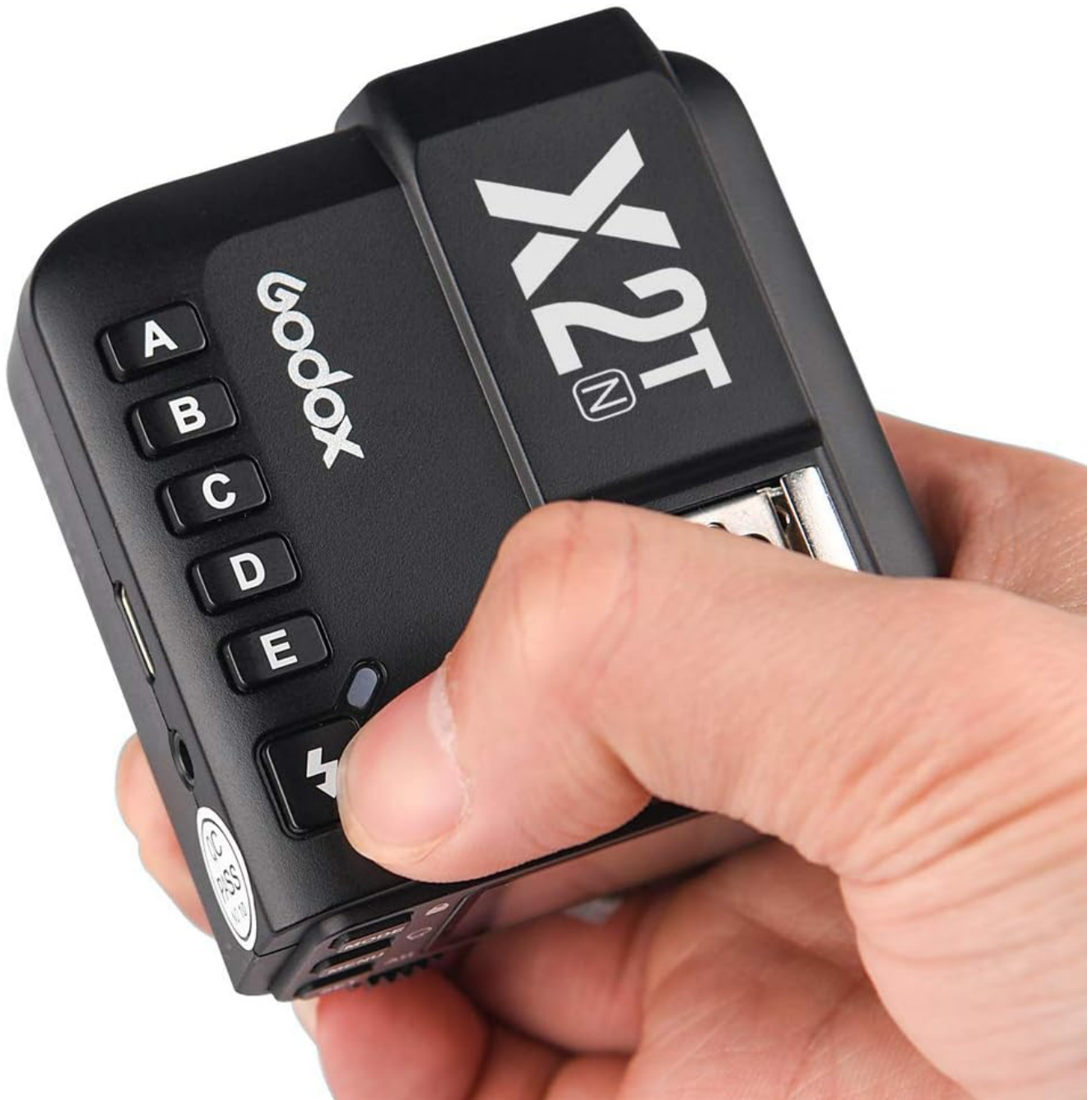
Image: A hand holding the Godox X2T-N, illustrating the placement of the group selection buttons (A, B, C, D, E) on the left side of the unit.
