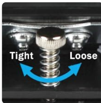
Figure 8: Adjusting screw for bill feeding tension.
