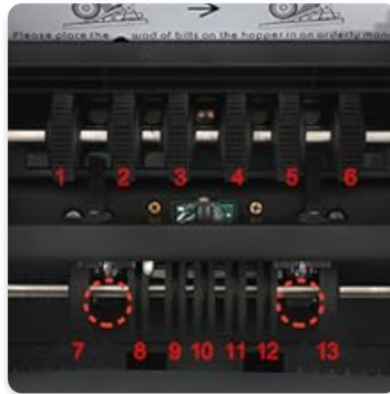
Figure 7: Internal rubber wheels and covered sensors.
