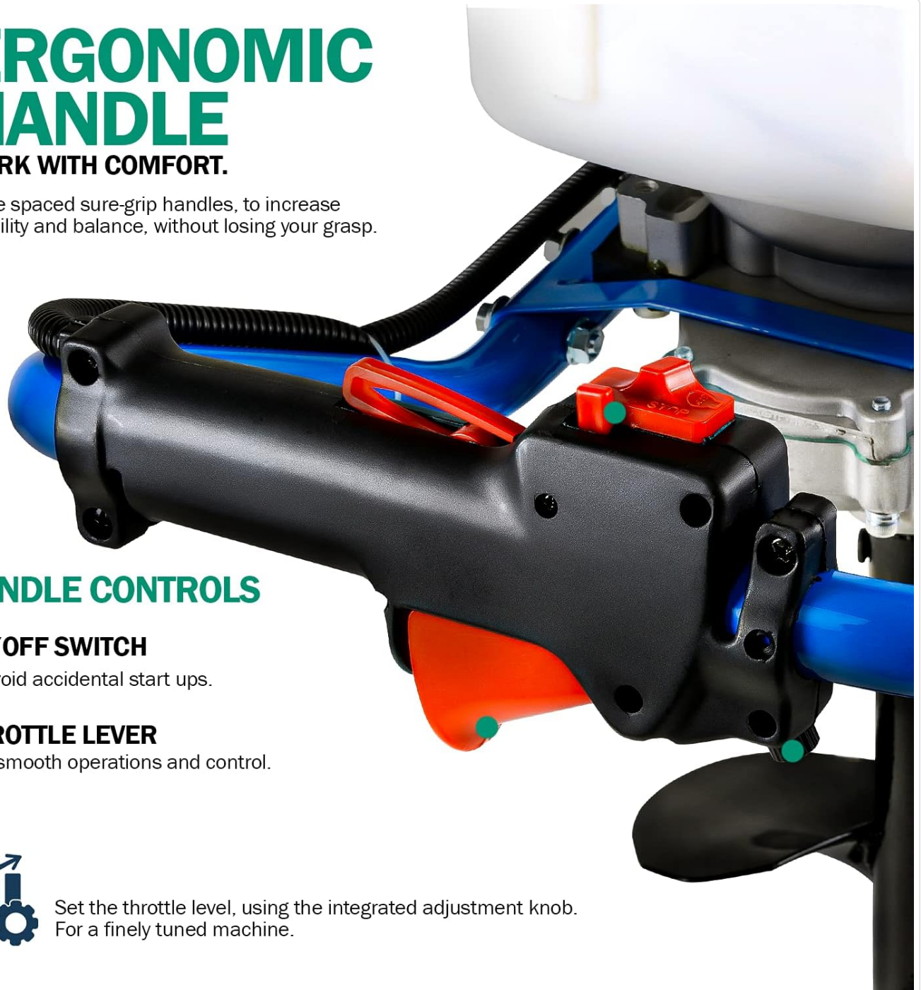
Figure 2.1: Ergonomic handle with ON/OFF switch and throttle lever for comfortable and controlled operation.
