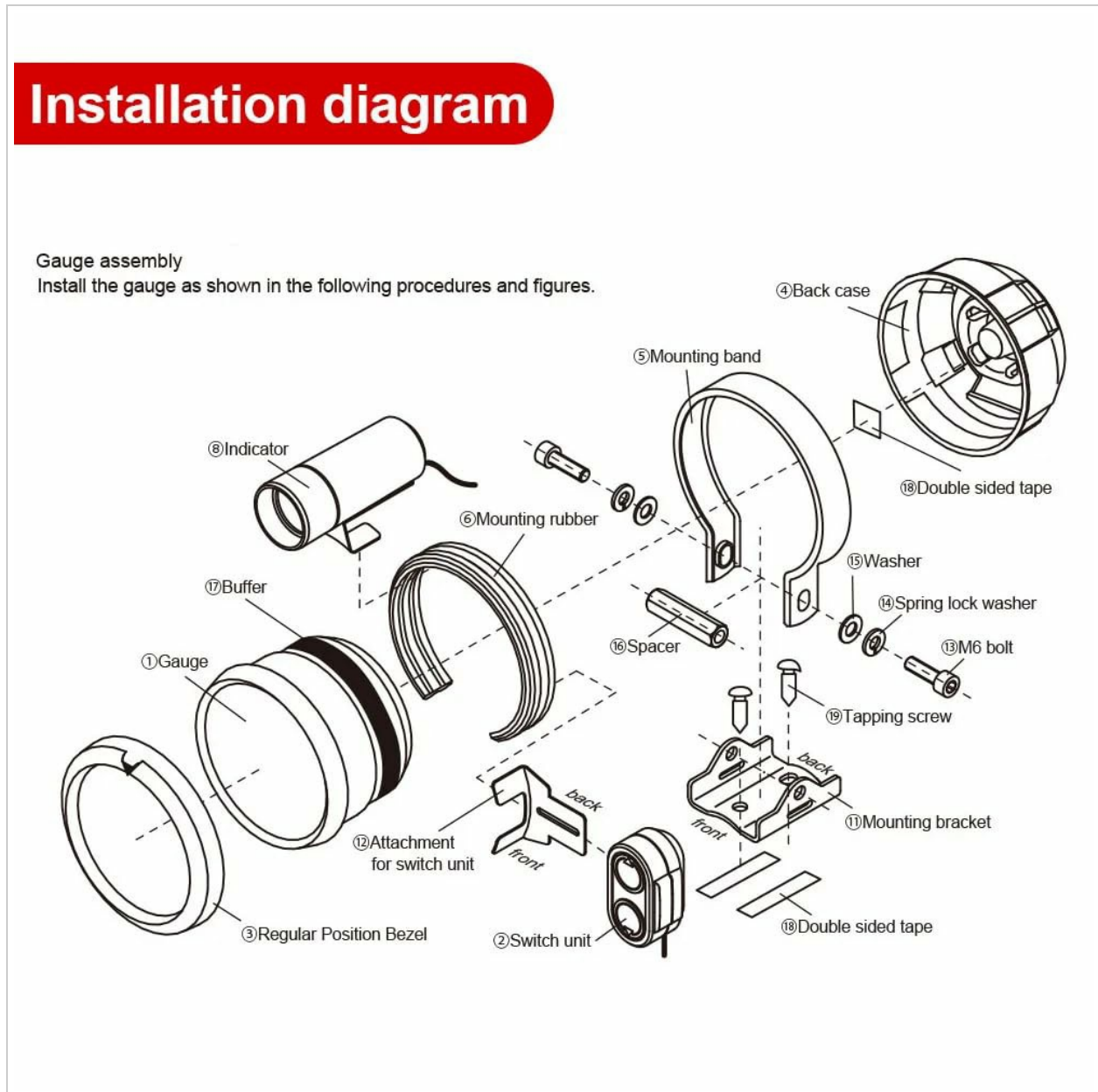
Image 5.1: Exploded view diagram illustrating the assembly of the tachometer components, including the gauge, mounting band, back case, switch unit, indicator, and various fasteners.
