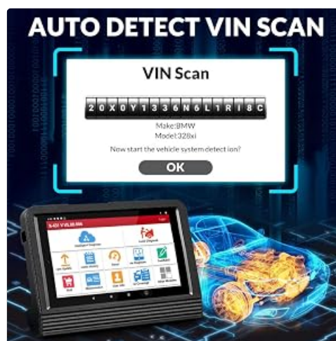
Image 3.1: The Auto VIN feature automatically detects vehicle identification numbers for quick and accurate diagnostics.
