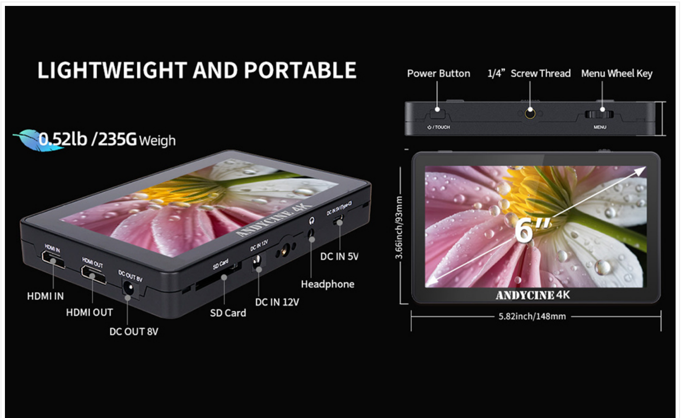
Image 3.2: Monitor ports and controls.
