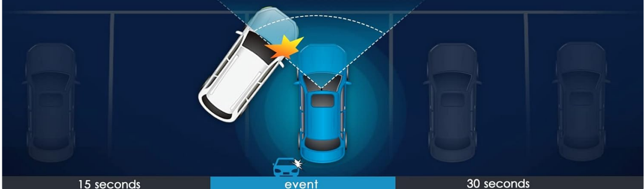
Figure 2.2: Illustration of the built-in GPS logger functionality and the three available parking modes: Auto Event Detection, Time Lapse Recording, and Low Bitrate Recording.
