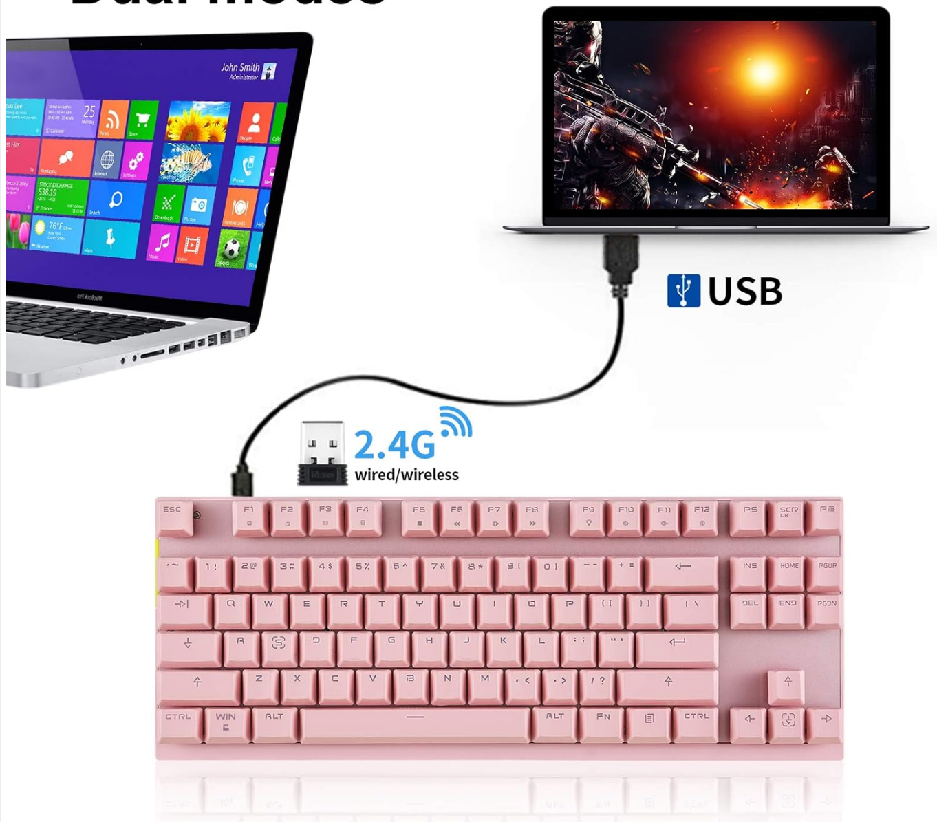
Image: The MOTOSPEED GK82 keyboard demonstrating its dual connectivity modes: wired via USB cable to a laptop and wireless via a 2.4G USB receiver to another laptop.
