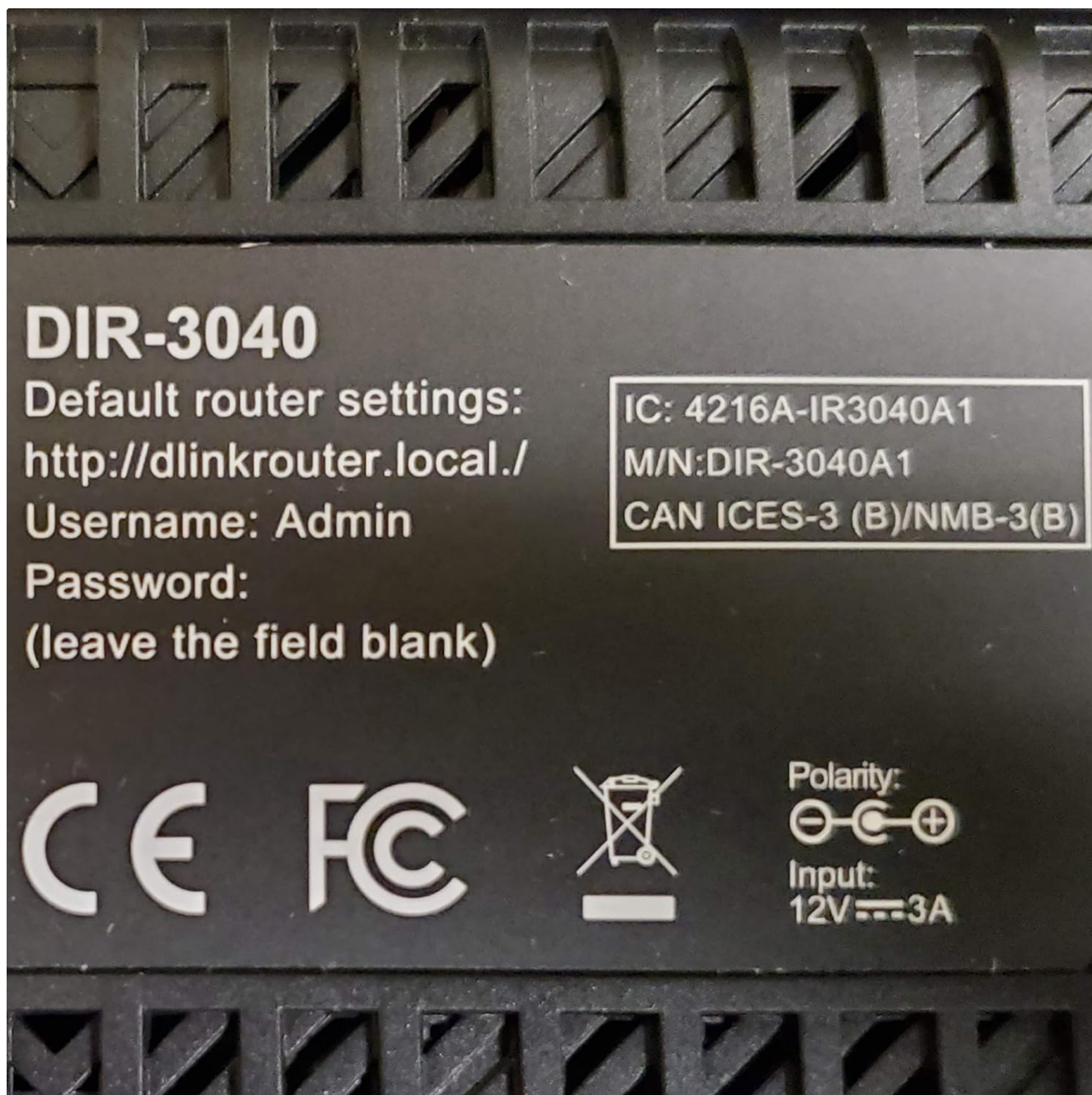
Figure 3: Bottom label of the D-Link DIR-3040 Router, displaying default router settings including the web address, username, and password information.
